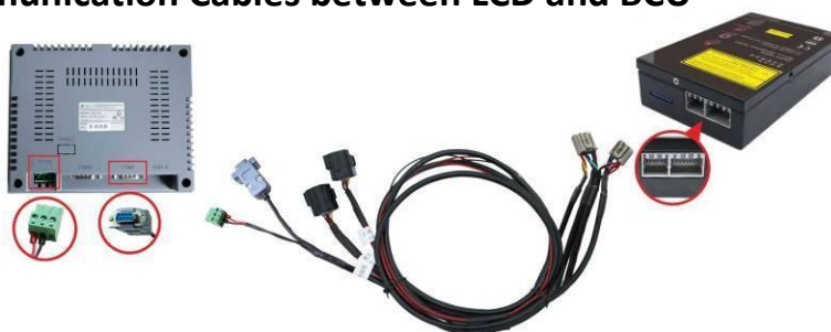
Figure 2-28 Example Diagram of Communication Cables between LCD and BCU
