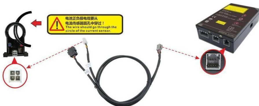
Figure 2-22 Example Diagram for Connection of Current Sensor
