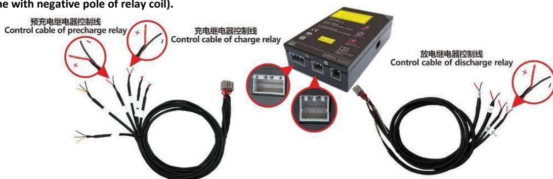
Figure 2-23 Example Diagram for Connection of Relay Control Cable
