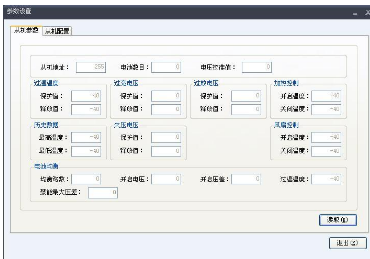
Figure 5-2 Display Interface 3 of Upper Computer Configuration
