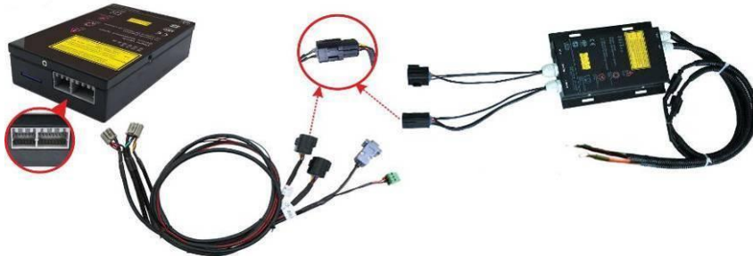
Figure 2-26 Example Diagram for Connection of Communication Cables between LDM and BCU
