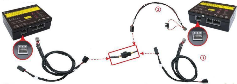
Figure 2-19 Example Diagram for Connection of Communication cables among BMUs
